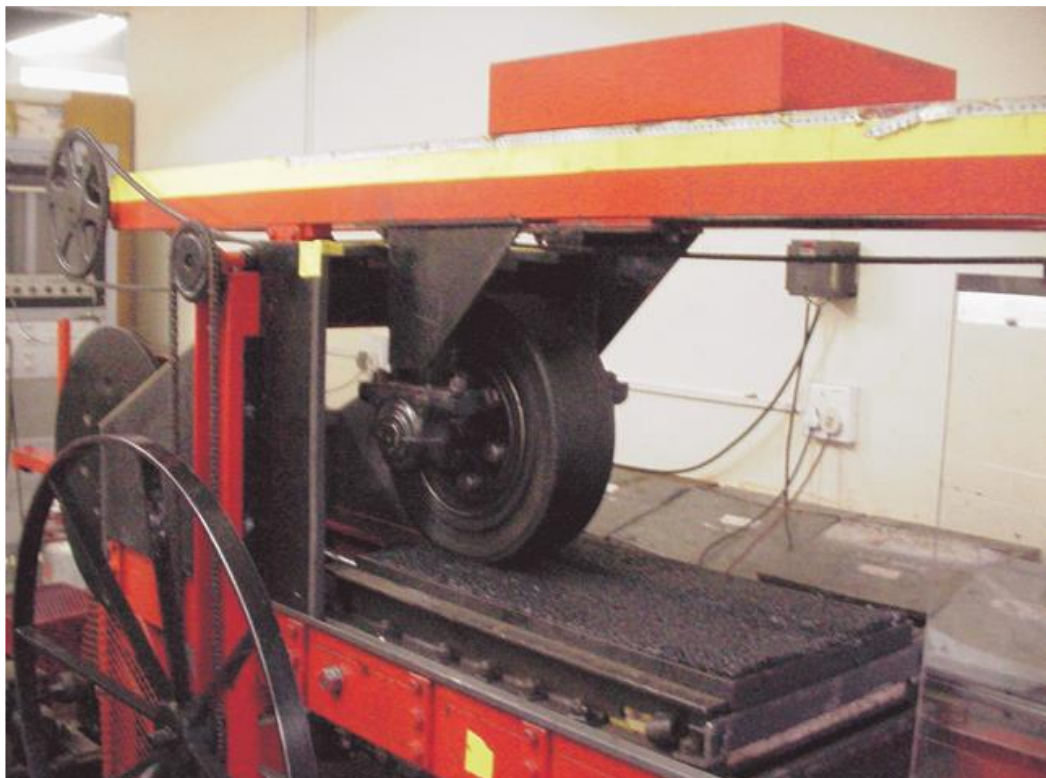
Figure C.2 — Compaction of Slab for Wheel Tracking Test
