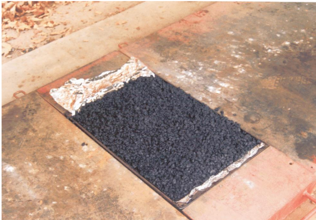
Figure C.6 — Compacted Sample using Rolling Wheel Compaction
