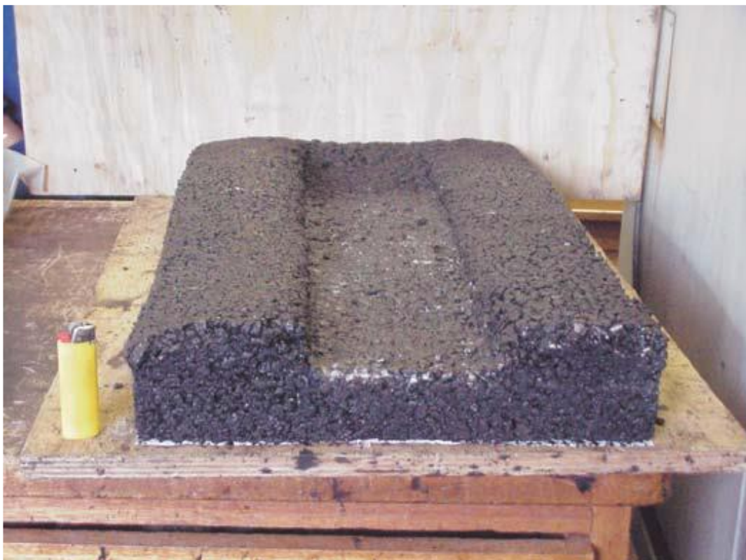
Figure C.4 — Deformation of Slab after a Wheel Tracking Test
