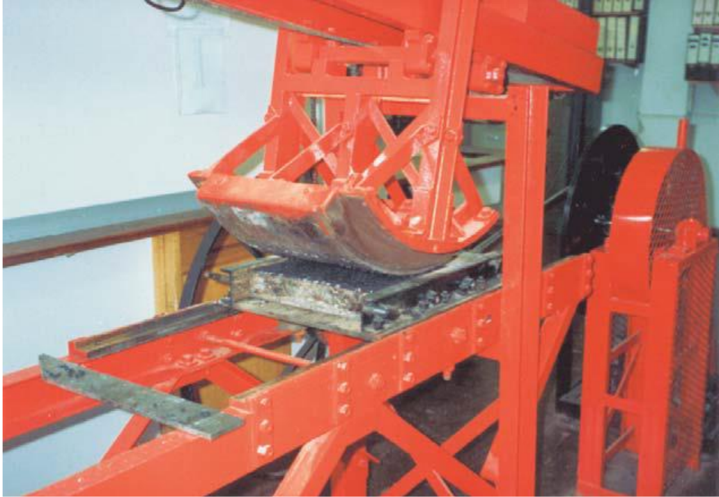
Figure C.2 — Compaction of Slab for Wheel Tracking Test
